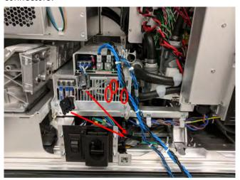
14. Loosen the three screws securing the power supply.
