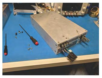
Attach the new brackets to the 48V power supply.
