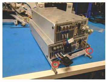
10. Push the grommet down making sure it covers the handle bracket and the small 90° bend from the left side bracket.
