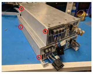
9. Reuse the old handle bracket with the grommet still partially attached and secure with the two screws.
