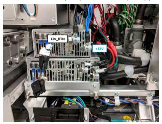
5. Connect the communication cables to each power supply.
