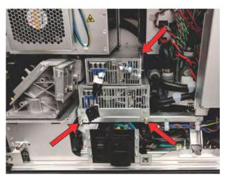
18. Remove the power supply assembly by sliding it out toward the back of the projector. Both power supplies are removed together. Slightly tilting the handle up and down as the assembly is removed can help slide it out.
