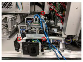
15. Remove the power supply assembly by sliding it out toward the back of the projector. Both power supplies are removed together. Slightly tilting the handle up and down as the assembly is removed can help slide it out.
