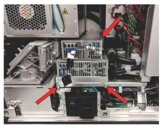
3. Attach the +48V (red) and 48 V\_RTN (black) power harness to the bottom power supply.
