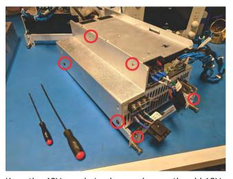
5. Keep the 48V supply in place and move the old 12V supply and brackets out of the way.
